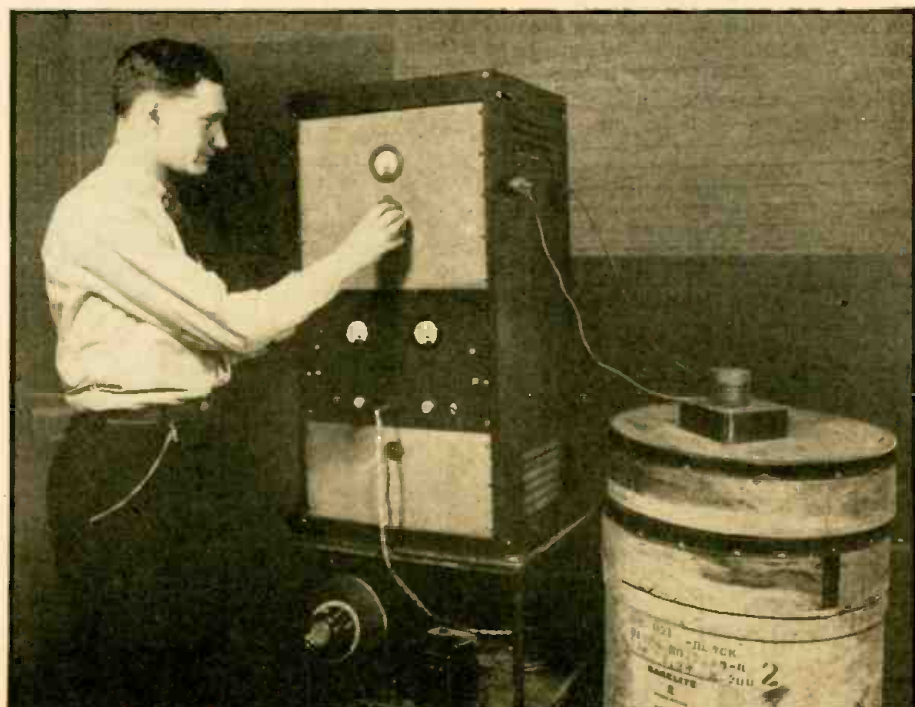
This compact and easily adjusted unit supplies all the heat necessary, and supplies it only at the point where it is used. Nothing is heated but the plastic and the plates which contact it.
