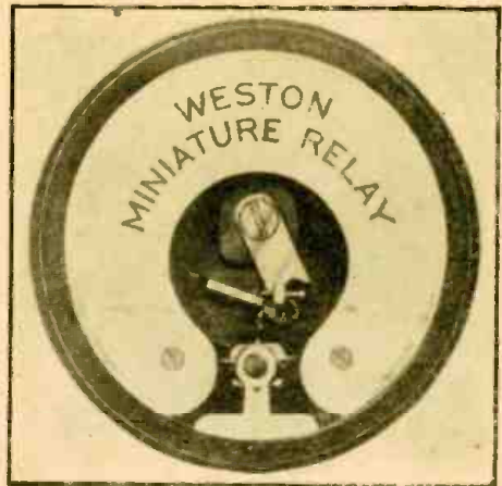
Sensitive milliammeter designed to work with electronic tubes. 200 microamperes applied to this relay will close contacts permitting up to 30 milliamperes, to flow in a local circuit.
